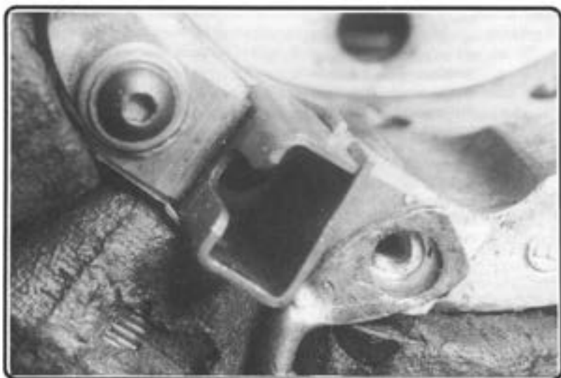
Figure 32. Brush-holder mounting screws and insulation.
