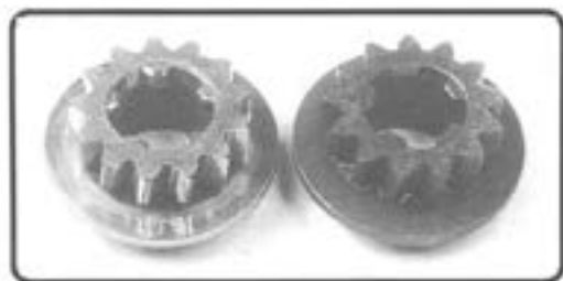
Figure 18. Small sliding gear.
