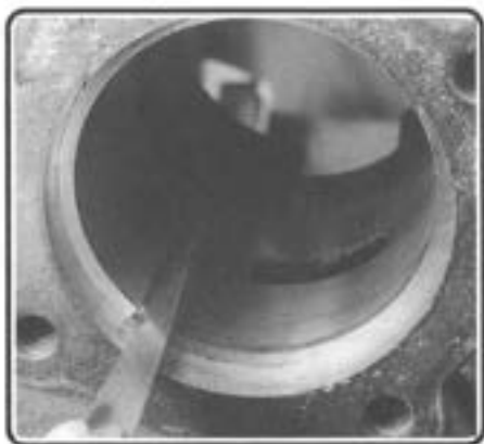
Figure 42. Measuring piston ring gap.
