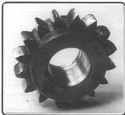
Figure 23. Scored driving sprocket.
