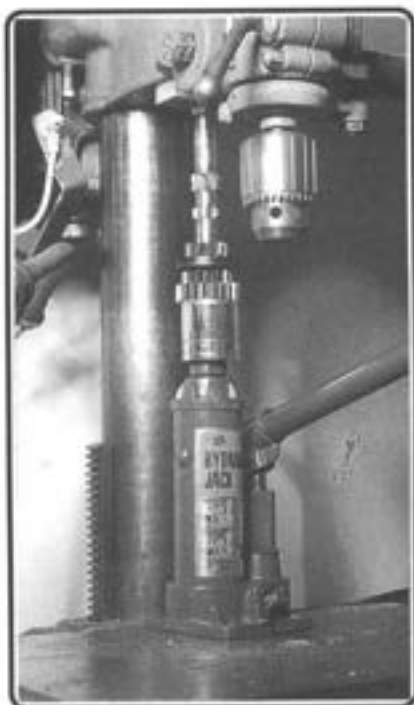
Figure 27. Pressing gear onto layshaft.
